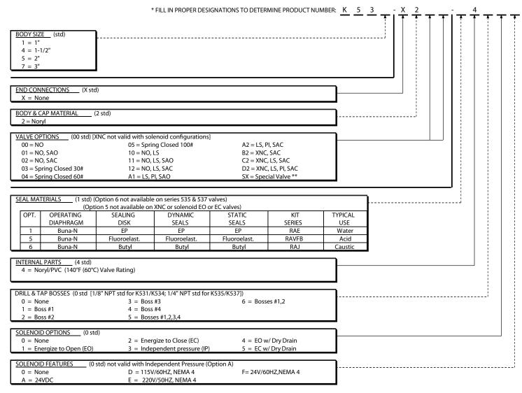
$^{*}$  To create a valve number replace each "\_" with the proper number or letter for the feature you desire.
